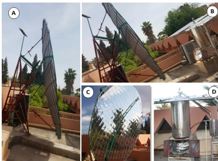
Figure 12. Solar distillation apparatus. (A and C) solar reflector; (B) solar apparatus; (D) distillation unit.
