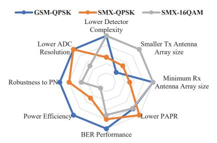
**Figure 3.35** – Comparison of MIMO Systems in sub-THz channels. Axes are normalized by the best achieved value among the 3 systems of same spectral efficiency.
