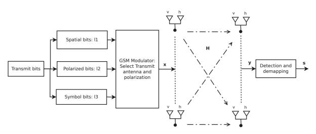
**Figure 3.28** –  $N_r \times N_t$  DP-GSM system model.
