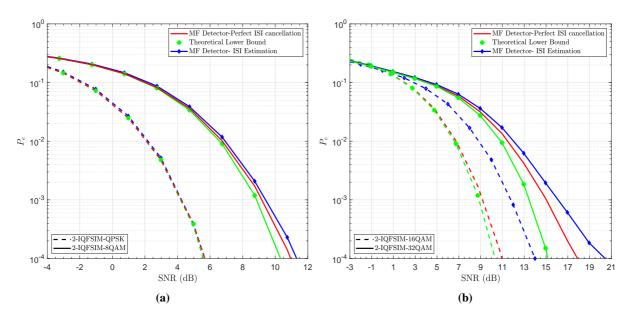
**Figure 4.22** – The error probabilities of filter index detection on I and Q with ISI estimation and cancellation, perfect ISI cancellation, and the derived theoretical lower bound, N = 2 (2-IQ-FSIM-MQAM). The SE is: (a) [4, 5] bits/symbol using M = [4, 8], (b) [6, 7] bits/symbol using M = [16, 32].
