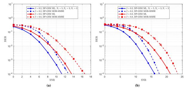
**Figure 3.29** – BER performance of  $N_r \times N_t$  DP-GSM system with spatial correlation  $\beta \in \{0.2, 0.8\}$  and power leakage parameter  $\mu = 0.2$  for QPSK over: (a) correlated Rayleigh channel and (b) correlated Rician channel (K = 3) using both MOB-MMSE and ML detectors. The spectral efficiency is 12 bpcu.
