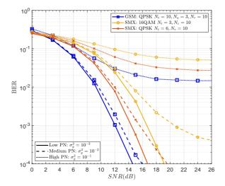
**Figure 3.17** – Average BER performance of 12bpcu MIMO SMX and GSM systems subjected to different phase noise levels in DO setup. AP-UE mean distance is  $d_{mean} = 5m$ . URA array geometry with  $4\lambda$  antenna separation is used with  $N_r = 10$ .
