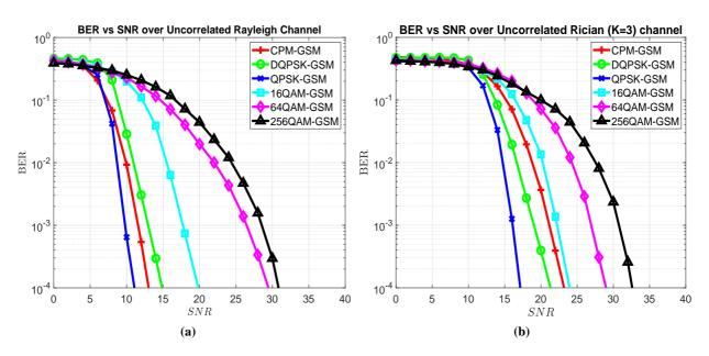
**Figure 3.3** – BER vs SNR for various APM-GSM systems over uncorrelated: (a) Rayleigh channel, (b) Rician channel.
