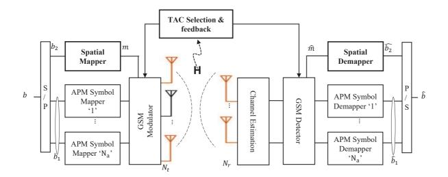
Figure 3.7 – System model of GSM with TAC selection
