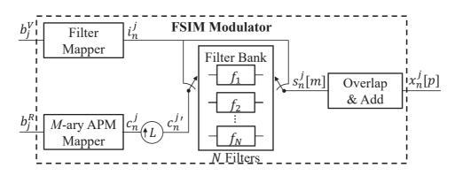
Figure 4.29 – System model of FSIM Modulator with *M*-ary APM mapping and a filter bank of *N* filters.
