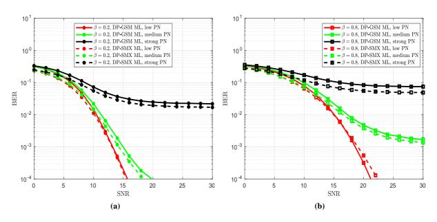
**Figure 3.32** – BER performance of DP-GSM and DP-SMX systems for QPSK over correlated Rician channel (K = 3) with spatial correlation: (a)  $\beta = 0.2$  and (b)  $\beta = 0.8$  using ML detector. Both systems are affected by PN with different levels (low, medium and strong noise). The power leakage parameter is  $\mu = 0.2$  and the spectral efficiency is 12 bpcu.
