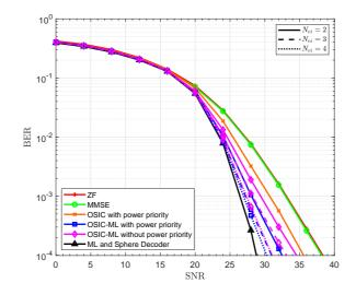
**Figure 3.22** – Uncoded BER performance of SMX-MIMO system using different detectors. The system parameters are: 64–QAM,  $N_t = 4$ ,  $N_r = 5$ ,  $N_{ei} = 2$ , 3 and 4 that has a spectral efficiency of 24 bpcu.
