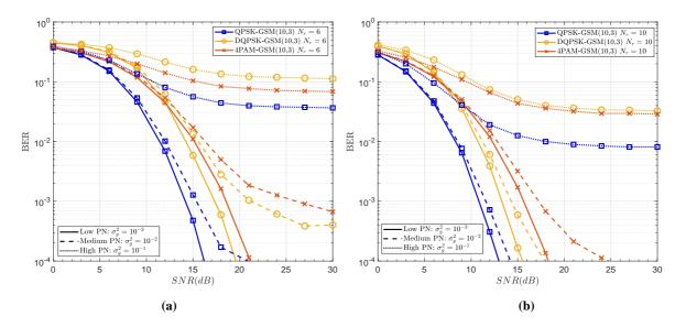
**Figure 3.14** – BER performance of different APM-GSM systems in sub-THz channels and with different PN levels in DO setup. The spectral efficiency is 12bpcu. The concerned sub-THz indoor MIMO channels are generated using ULA array geometry with  $4\lambda$  antenna separation. (a)  $N_r = 6$ , (b)  $N_r = 10$ .
