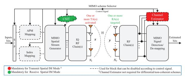
Figure 2.5 – General system model for MIMO system with/without spatial IM.
