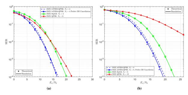
**Figure 4.31** – SER performance of the proposed SMX 2-FSIM-QPSK system and its equivalent SMX-QAM systems of the same SE: (a) SE= 12 bpcu with  $N_r = 8$ , (b) SE= 24 bpcu with  $N_r = 12$ .
