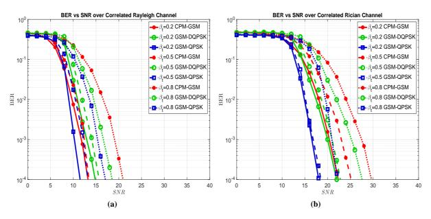
**Figure 3.4** – BER vs SNR for (D)QPSK-GSM and CPM-GSM over correlated: (a) Rayleigh channel, (b) Rician channel.
