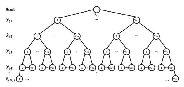
**Figure 3.20** – The tree search for the OSIC-ML MIMO detectors of  $N_t$  height and  $N_{ei}$  branching factor. The corresponding branches of each node in the tree are numbered from 1 to  $N_{ei}$ .
