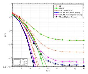
**Figure 3.24** – Uncoded BER performance of SMX-MIMO system using different detectors with perfect and imperfect channel estimation. The system parameters are: QPSK,  $N_t = 6$ ,  $N_r = 10$ ,  $N_{ei} = 2$  and  $\sigma_e^2 = [0, 10^{-2}, 10^{-3}]$ . The SE is 12 bpcu.
