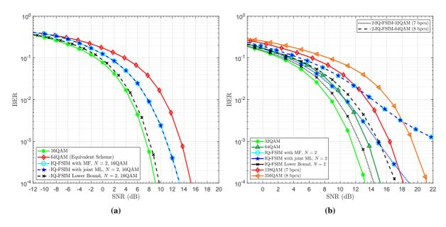
**Figure 4.24** – Uncoded BER performance of 2-IQ-FSIM-*M*QAM, its theoretical lower bound and its equivalent scheme 4*M*QAM of the same SE: (a) 6 bits/symbol using M = 16, (b) 7 and 8 bits/symbol using M = 32 and M = 64 respectively.
