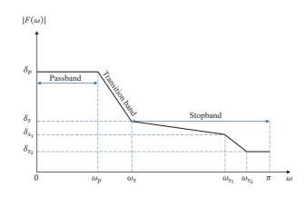
Figure 5.2 – A transmit spectral mask template.
