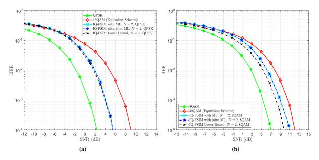
**Figure 4.23** – Uncoded BER performance of 2-IQ-FSIM-MQAM, its theoretical lower bound and its equivalent scheme 4MQAM of the same SE: (a) 4 bits/symbol using M = 4, (b) 5 bits/symbol using M = 8.
