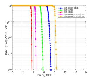
**Figure 4.35** – Comparison of CCDF of PAPR for the SMX FSIM, the SMX QAM and the GSM systems with pulse shaping having SE= 12 bpcu. SMX FSIM uses the filter shapes presented in [22], while SMX QAM and GSM use RRC filter.
