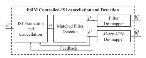
Figure 4.30 – System model of FSIM demodulator with the controlled-ISI cancellation and detection.
