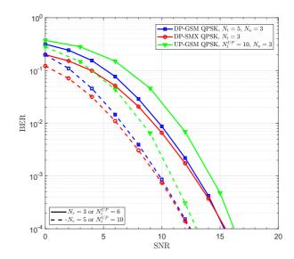
**Figure 3.33** – BER performance of DP-GSM , DP-SMX and UP-GSM systems with sub-THz channels and QPSK using ML detector.
