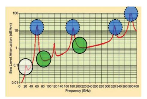
Figure 1.2 – Air attenuation at microwave, mmWave frequency bands [12, 13].
