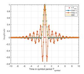
**Figure 4.21** – Complete responses of the 2 filters obtained after correct matched filtering at the receiver side, where  $\eta = 10$  and  $\lambda = 8$ .
