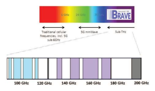
Figure 1 – Frequency allocation for wireless communications in BRAVE considered spectrum [4].
