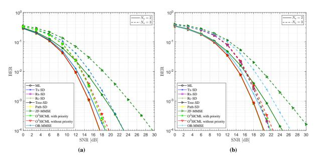
**Figure 3.25** – Uncoded GSM performance with  $N_t = N_r = 5$  and  $N_a = [2, 3]$  and different linear and non-linear detectors: (a) 16QAM, (b) 32QAM
