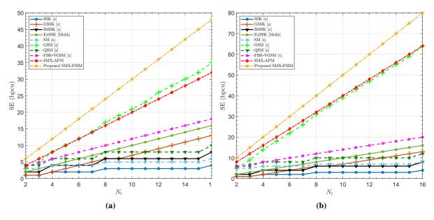
**Figure 4.33** – Maximum SE for different MIMO techniques:  $N_a = [1, ..., N_t - 1]$  for fixed  $N_a$  schemes, N = 2 for FSIM, and different *M* for systems with APM: (a) M = 4, (b) M = 16.
