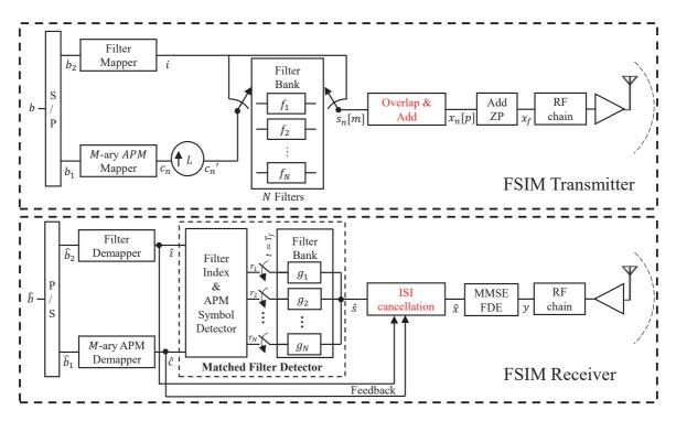
**Figure 4.1** – System model of the FSIM-based transmitter and receiver with MF-based detector using N filters of length L and M-ary APM. Note that the detector can be replaced by the joint ML detector.
