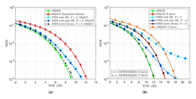
**Figure 4.10** – Uncoded BER performance of 2-FSIM-MQAM, its analytical lower bound and its equivalent scheme 2MQAM of the same SE: (a) 5 bits/symbol using M = 16, (b) 6 and 7 bits/symbol using M = 32 and M = 64 respectively.
