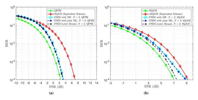
**Figure 4.9** – Uncoded BER performance of 2-FSIM-MQAM, its analytical lower bound and its equivalent scheme 2MQAM of the same SE: (a) 3 bits/symbol using M = 4, (b) 4 bits/symbol using M = 8.
