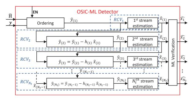
**Figure 3.19** – OSIC-ML model with/without ordering. 'EN' is a boolean variable to activate the ordering technique prior to detection and interference cancellation. The stream estimator in the  $N_t$  receive circuits is based on a linear symbol detection.
