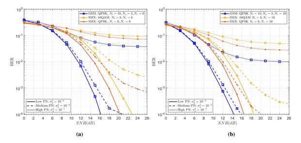
**Figure 3.16** – Average BER performance of 12bpcu MIMO SMX and GSM systems subjected to different phase noise levels in DO setup. AP-UE mean distance is  $d_{mean} = 5m$ . ULA array geometry with  $4\lambda$  antenna separation is used with (a)  $N_r = 6$ , (b)  $N_r = 10$ .
