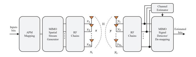
Figure 2.4 – MIMO transceiver System Model with  $N_t$  transmit antennas and  $N_r$  receive antennas.
