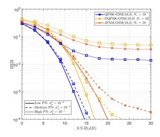
**Figure 3.15** – BER performance of different APM-GSM systems in sub-THz channels and with different PN levels in DO setup. The spectral efficiency is 12bpcu. The concerned sub-THz indoor MIMO channels are generated using URA array geometry with  $4\lambda$  antenna separation and  $N_r = 10$ .
