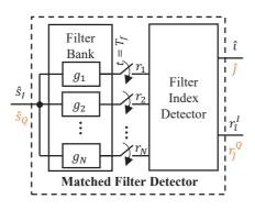
**Figure 4.16** – Matched filter detector with input either  $\hat{s}^I$  or  $\hat{s}^Q$  to detect the index of the used filter shape  $\hat{i}$  or  $\hat{j}$  respectively.
