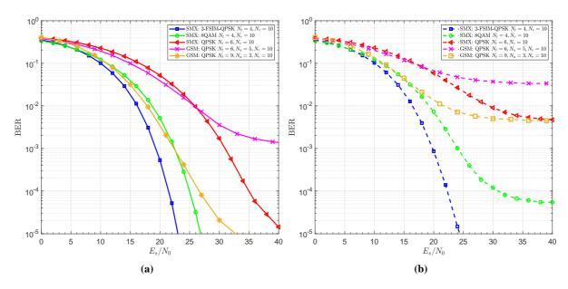
**Figure 4.34** – Uncoded BER performance of the proposed non-coherent SMX FSIM compared to SMX-QAM and GSM in sub-THz channels. The SE for all systems is 12 bits/symbol (bcpu) and they are subjected to different PN levels: (a) low PN ( $\sigma_g^2 = 10^{-1}$ ), (b) medium PN ( $\sigma_g^2 = 10^{-2}$ ).
