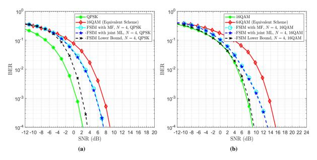
**Figure 4.13** – Uncoded BER performance of 4-FSIM-MQAM, its analytical lower bound and its equivalent scheme 4MQAM of the same SE: (a) 4 bits/symbol using M = 4, (b) 6 bits/symbol using M = 16.
