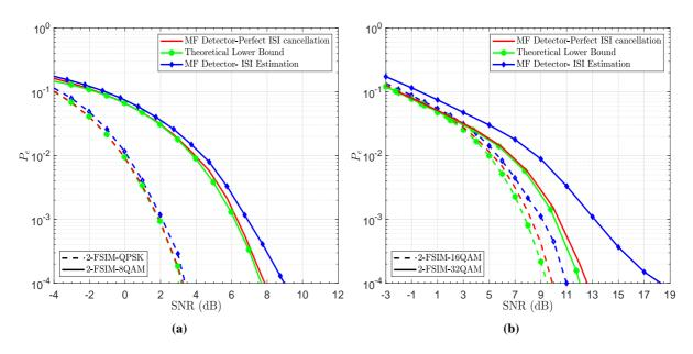
**Figure 4.8** – The error probabilities of filter index detection with ISI estimation and cancellation, perfect ISI cancellation, and the derived theoretical lower bound, N = 2 (2-FSIM-*M*QAM). The SE is: (a) [3, 4] bits/symbol using M = [4, 8], (b) [5, 6] bits/symbol using M = [16, 32].
