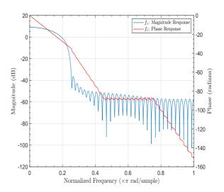
**Figure 4.5** – Magnitude and phase response of the filter  $f_1$  depicted in Fig. 4.4.
