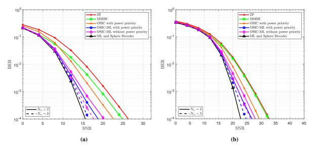
**Figure 3.21** – Uncoded BER performance of SMX-MIMO system using different detectors. The system parameters are:  $N_t = 4$ ,  $N_r = 5$ ,  $N_{ei} = 2$  and 3: (a) QPSK (SE=8 bpcu), (b) 16–QAM (SE=16 bpcu).
