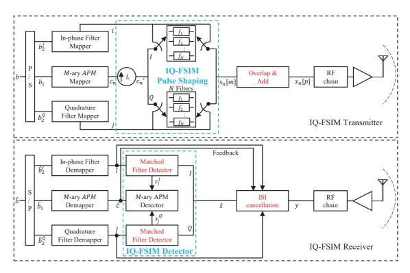
**Figure 4.15** – System model of the IQ-FSIM based transceiver with MF-based detector using N filters of length L and M-ary APM. Note that the joint ML detector can replace the IQ-FSIM detector.
