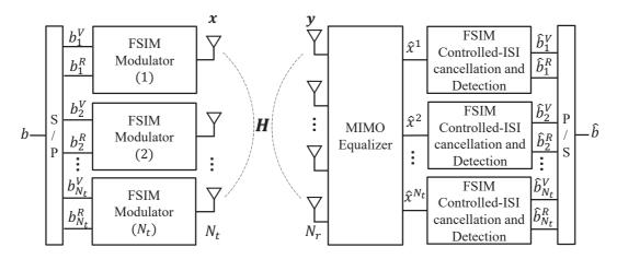
**Figure 4.28** – System model of  $N_t \times N_r$  SMX-FSIM transceiver.
