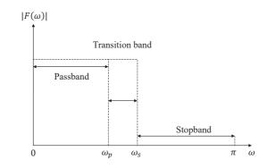
Figure 5.1 – Low pass filter magnitude response.
