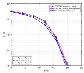
**Figure 3.23** – Uncoded BER performance of SMX-MIMO system using different detectors with different number of TAs. The system parameters are: 16–QAM,  $N_t = [4, 6, 8]$ ,  $N_r = N_t + 2$ ,  $N_{ei} = 4$ . The SE is [16, 24, 32] bpcu.
