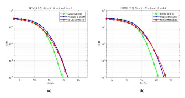
**Figure 3.8** – BER vs  $E_b/N_0$  for various TAC selection with: (a)  $\beta_t = 0$ , (b)  $\beta_t = 0.4$ .
