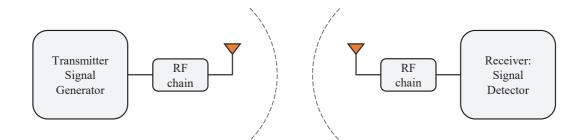
Figure 2.3 – General SISO wireless communication sytem.
