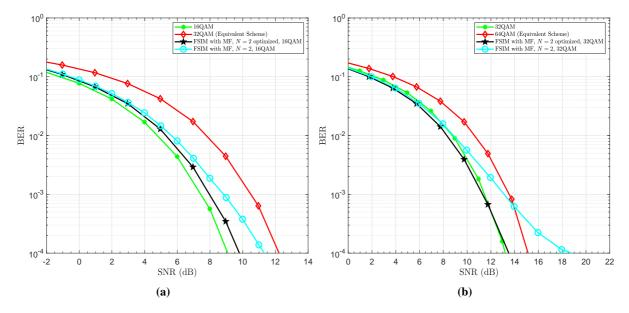
**Figure 5.6** – Uncoded BER performance of 2-FSIM-MQAM with optimized filter shapes, and its equivalent scheme 2MQAM of the same SE: (a) 5 bits/symbol using M = 16, (b) 6 bits/symbol using M = 32.
