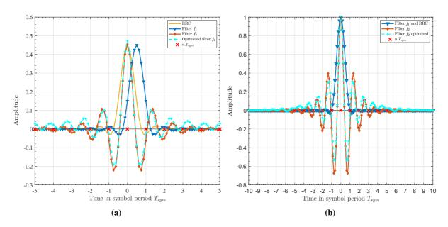
**Figure 5.4** – Comparison of the previous intuitive filters and the optimized filter  $f_2$  using the iterative ISI minimization in Algorithm 4: (a) impulse responses, (b) complete responses after correct matched filtering at the receiver side.
