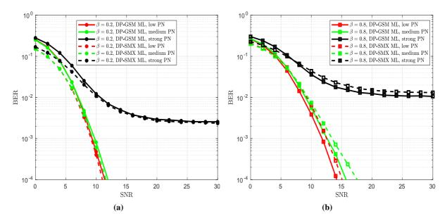
**Figure 3.31** – BER performance of DP-GSM and DP-SMX systems for QPSK over correlated Rayleigh channel with spatial correlation: (a)  $\beta = 0.2$  and (b)  $\beta = 0.8$  using ML detector. Both systems are affected by PN with different levels (low, medium and strong noise). The power leakage parameter is  $\mu = 0.2$  and the spectral efficiency is 12 bpcu.
