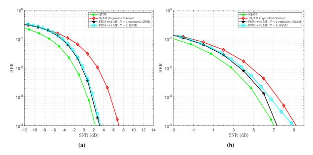
**Figure 5.5** – Uncoded BER performance of 2-FSIM-MQAM with optimized filter shapes, and its equivalent scheme 2MQAM of the same SE: (a) 3 bits/symbol using M = 4, (b) 4 bits/symbol using M = 8.
