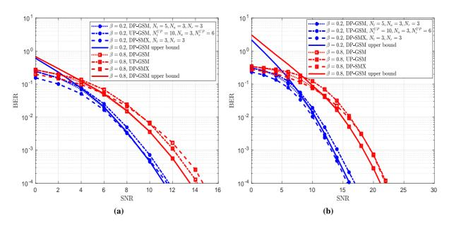
**Figure 3.30** – BER performance comparison of DP-GSM , DP-SMX, and UP-GSM systems with spatial correlation  $\beta \in \{0.2, 0.8\}$  and power leakage  $\mu = 0.2$  over: (a) correlated Rayleigh channel and (b) correlated Rician channel (K = 3) for QPSK using ML detector. The spectral efficiency is 12 bpcu.
