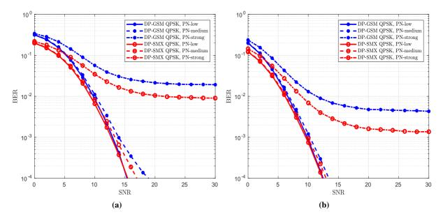
**Figure 3.34** – BER performance of DP-GSM and DP-SMX systems with sub-THz channels and different PN levels. The spectral efficiency is 12 bpcu.(a)  $N_r = 3$  and (b)  $N_r = 5$ .
