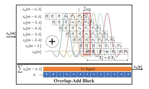
**Figure 4.2** – An example for the Overlap-Add block in the proposed scheme assuming  $\eta = 6$  symbols.
