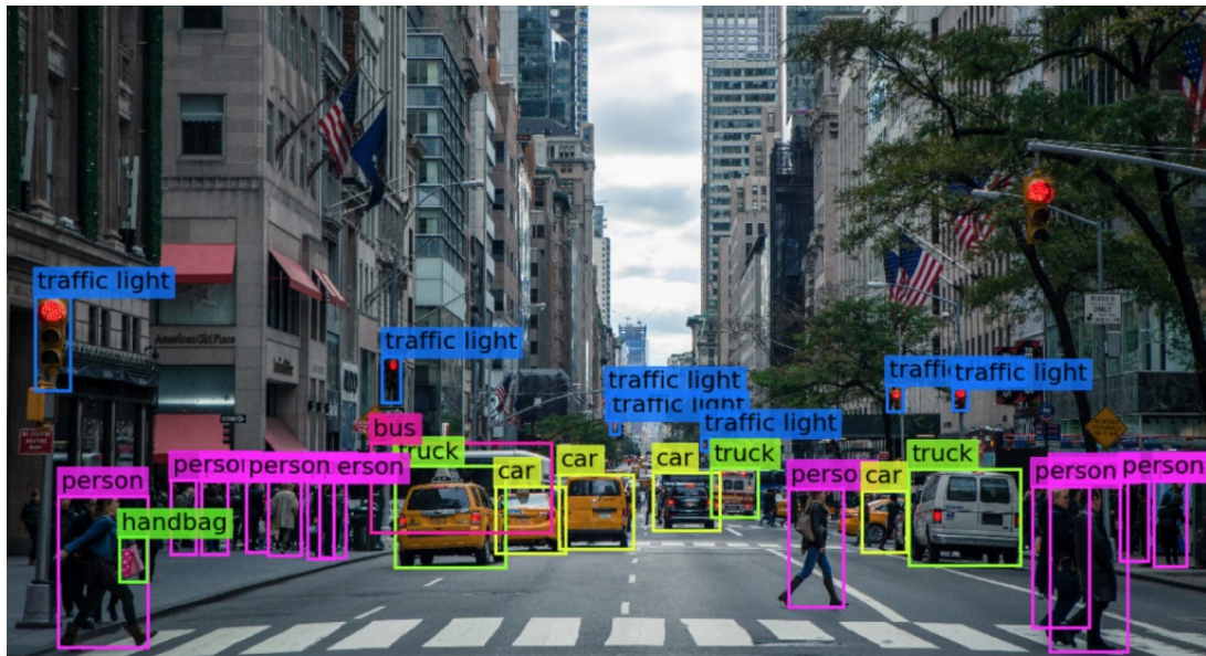
Figure 11.4: Image of the prediction of a computer vision deep learning algorithm for autonomous vehicle. Objects are classified based on a list of useful elements for driving and are localized into a boundary box. Image credits www.lebigdata.fr .
