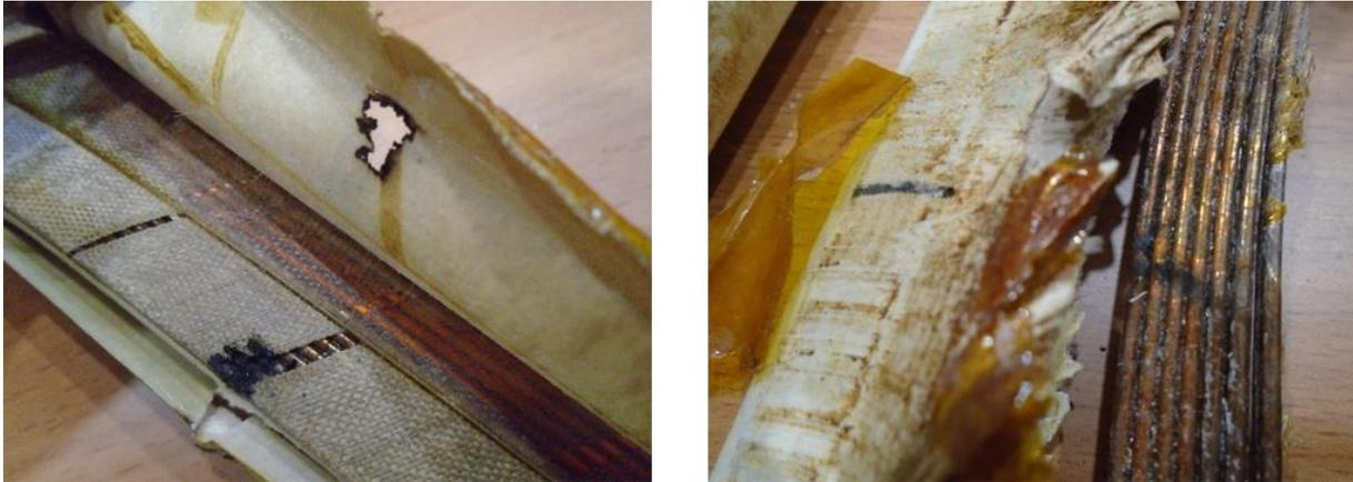
**Figure IV-19:** *Degradation of Type N phase-to-ground insulation systems subject to PDs*
