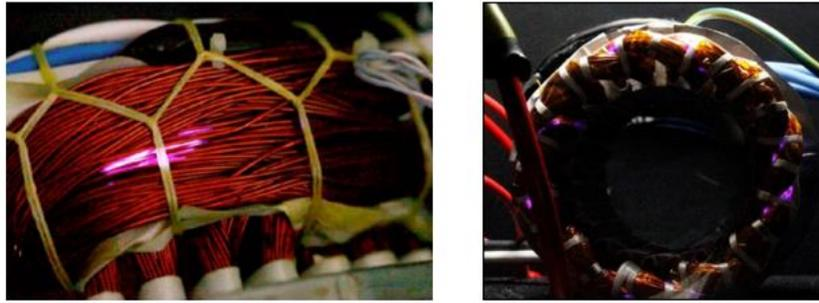
**Figure I-6:** *Manifestation of glow PDs in end-winding and probably between phases (left) and in the stator slot (right) [9]*
