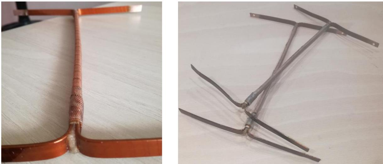
**Figure IV-1:** *Type II pairs of insulated conductors*
