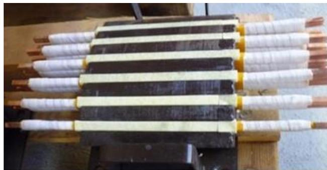
**Figure III-3:** Example of a phase-to-phase / phase-to-ground test sample
