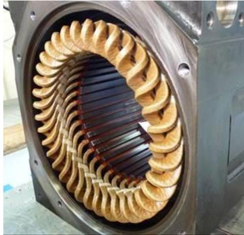
**Figure I-11:** *Insulation materials in the stator windings of a formed-wound machine*
