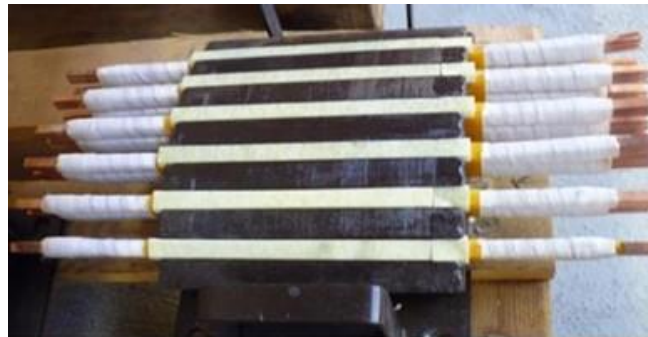
Figure III-3: Example of a phase-to-phase / phase-to-ground test sample
