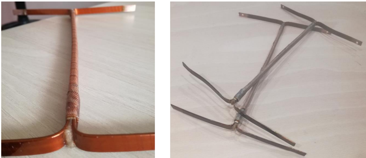
Figure IV-1: Type II pairs of insulated conductors
