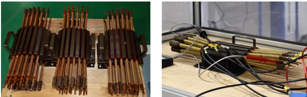
Figure IV-8: Morettes to study phase-to-phase and phase-to-ground insulation systems
