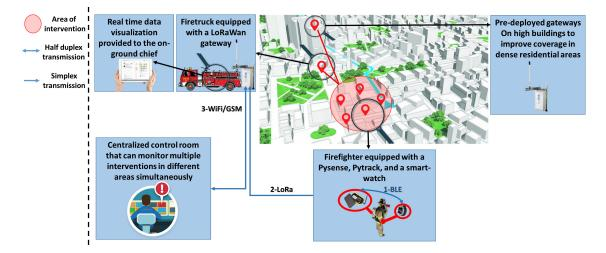
Figure 5.4: The proposed remote monitoring system
