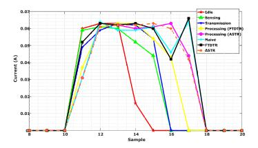
Figure 5.18: Peak current consumption comparison (LoRa)
