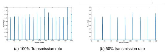
Figure 5.24: Current consumption times series comparison
