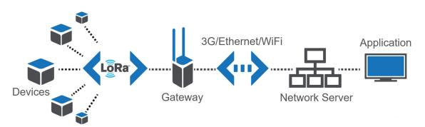
Figure 5.1: The LoRaWan network architecture
