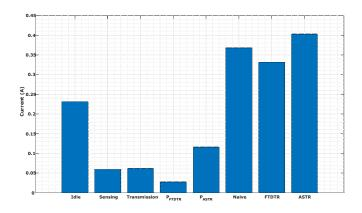
Figure 5.19: Peak current consumption comparison (LoRa)
