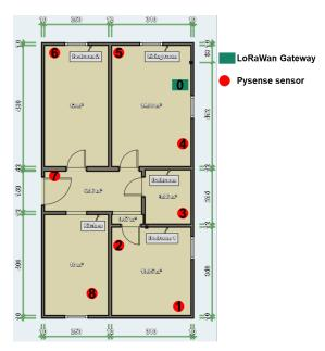
Figure 5.22: The sensor network geographical distribution
