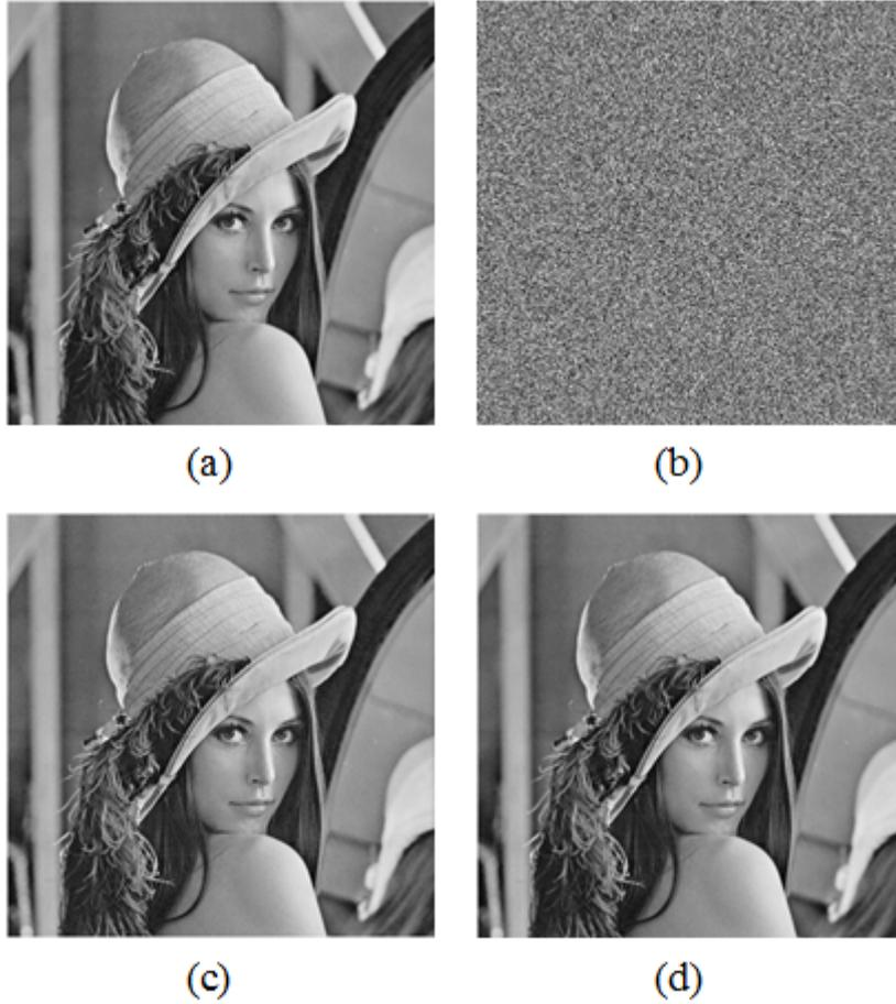
Figure 4.17: Simulation results of the proposed scheme on “Lena”: (a) original image; (b) watermarked-encrypted image, with  $\Delta = 3$  and message encoded with Hamming (7, 4) the error correction code; (c) decrypted-watermarked image where  $PSNR = 41 \text{ dB}$  and  $SSIM = 0.998$ ; (d) reconstructed image.
