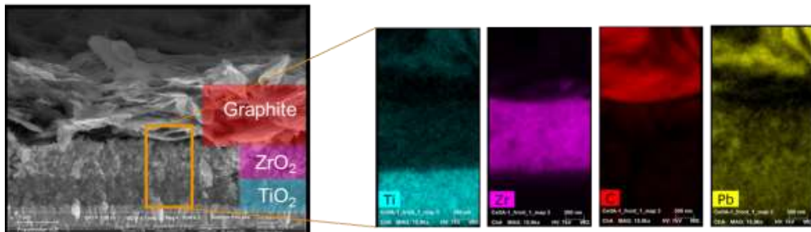
Figure III-24: SEM/EDX in mapping mode images of the complete cell after perovskite precursors infiltration in the porous layers
