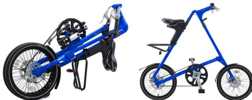
Figure 79: Foldable STRIDA bicycle folded (left), and unfolded (right)
