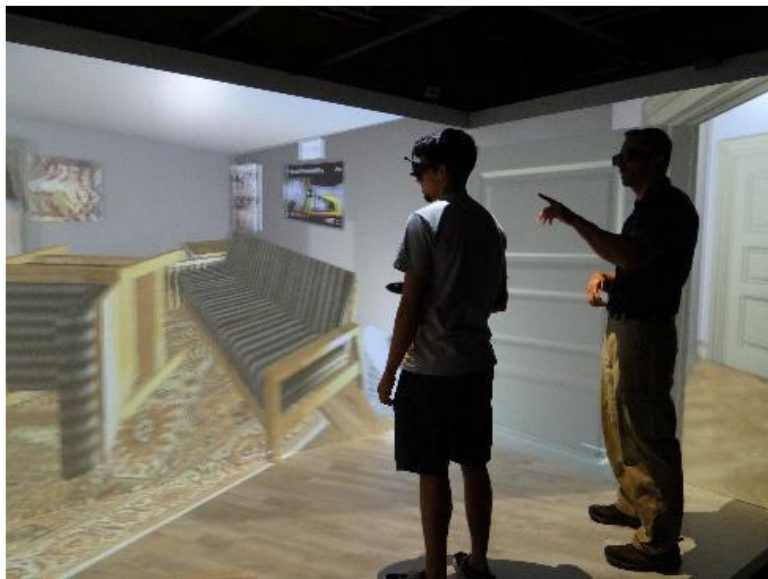
Figure 9: The Cave Automatic Virtual Environment (CAVE) (P. Marayong, et al., 2020)
