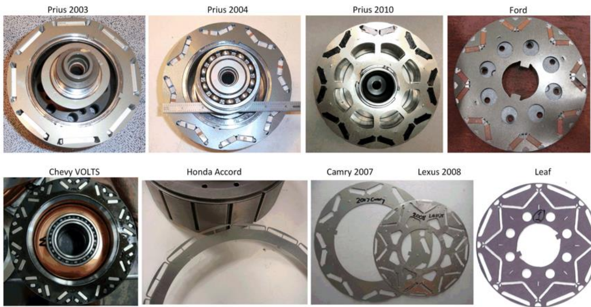
Figure 1.14 : Rotor laminations of different PM Machines in EV and HEV [23].
