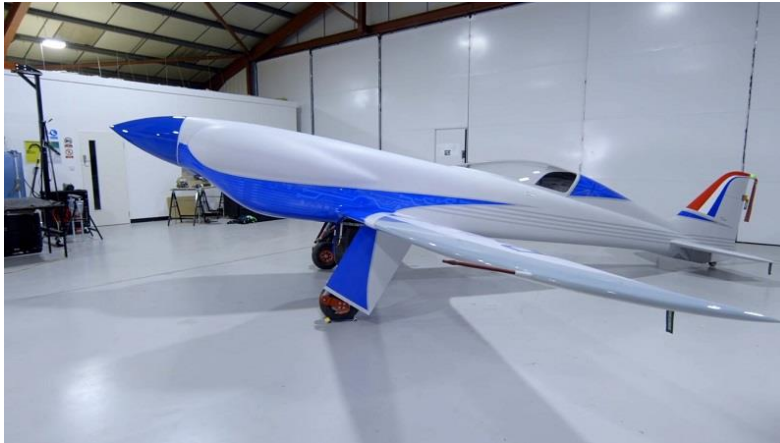
Figure 1.7 : ACCEL Iron Bird test airframe [9].
