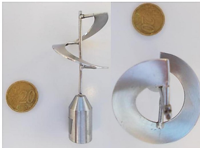
Figure 1.5: Lateral and top view of the impeller developed to measure the viscosity of filamentous suspensions (Hardy et al., 2015).
