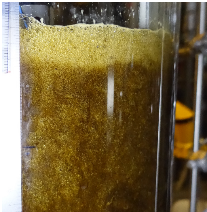
Figure 4.5: Presence of microbubbles in aerated broth.
