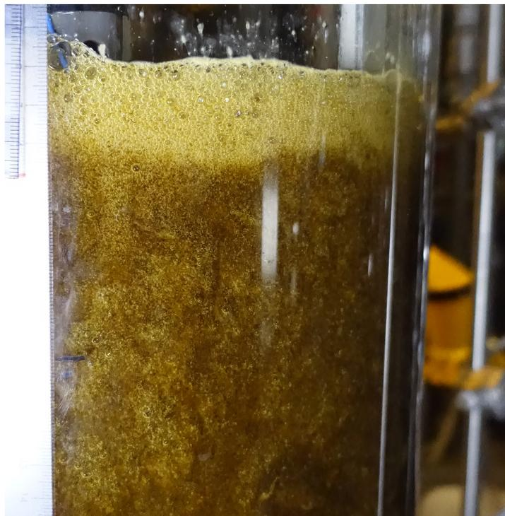
Figure 4.5: Presence of microbubbles in aerated broth.
