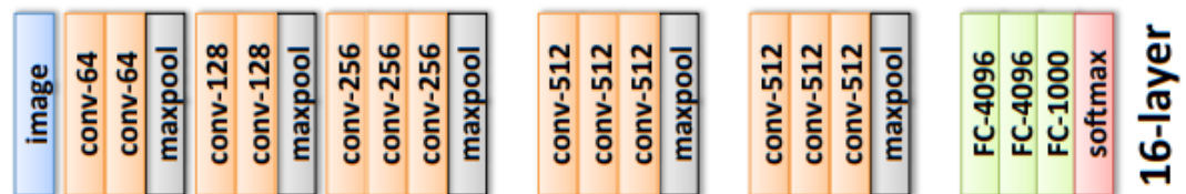
Figure 2.2: Network architecture of VGG-16 [96]
