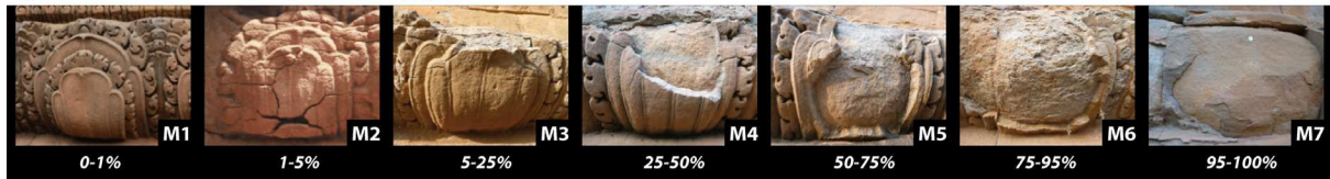
5-point scale of chemical weathering grades : visual assessment of matter loss
