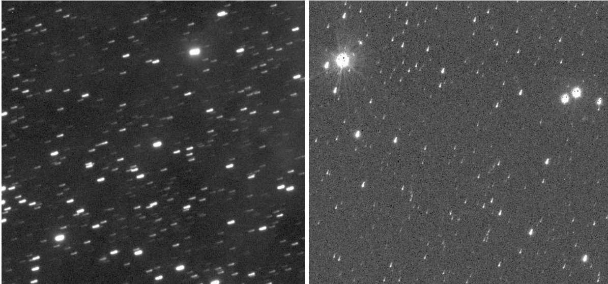
Figure 5.14: Left: tracking error in a CTIO-Mosaic2 image. Right: tracking error in a VISTA image.
