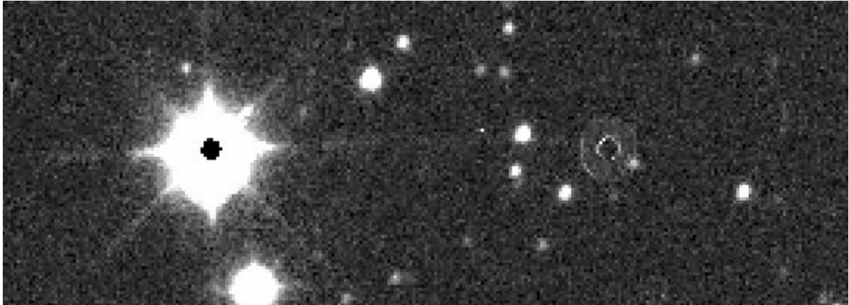
Figure 5.4: Example of a crosstalk pattern between channels in a WFCAM image.
