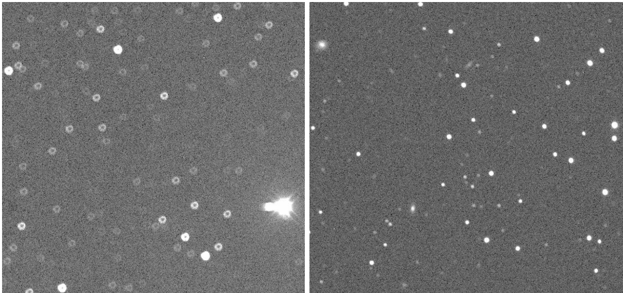
Figure 5.15: Left: defocusing in a KPNO-Mosaic1 exposure. Right: defocusing in a VIMOS exposure.
