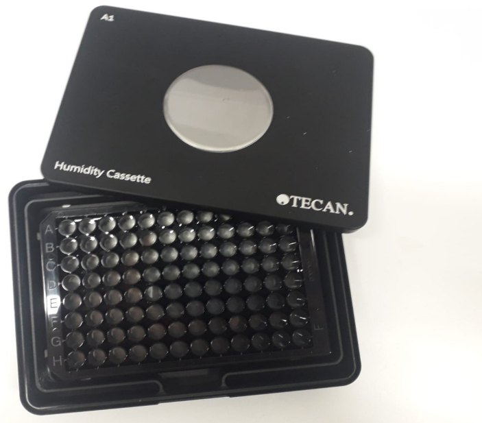
Figure 2.6: Humidity cassette. Picture credit: Chetan Aditya.
