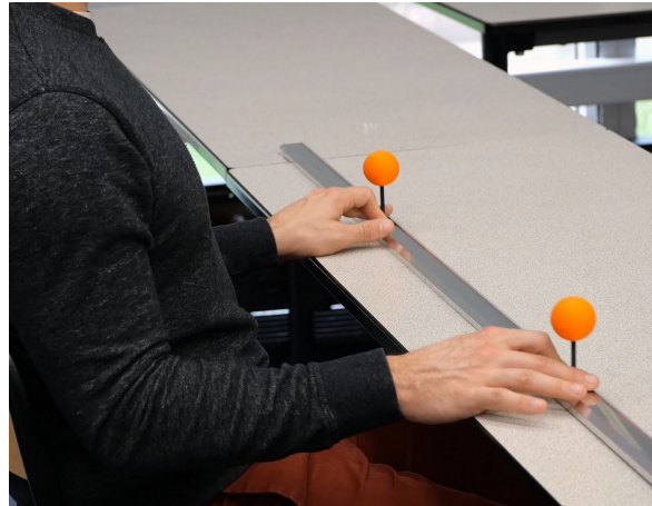
Figure 5.2 – Participants could provide the perceived exocentric distance by placing two sliding spheres. After the participants placed the spheres the system automatically took a picture of both spheres which was used to measure the distance between both spheres.
