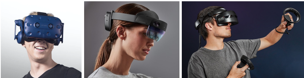
Figure 2.2 – Example of commercial HMDs: the HTC Vive (left), the Microsoft HoloLens 2 (center) and the HP VR1000 (right)
