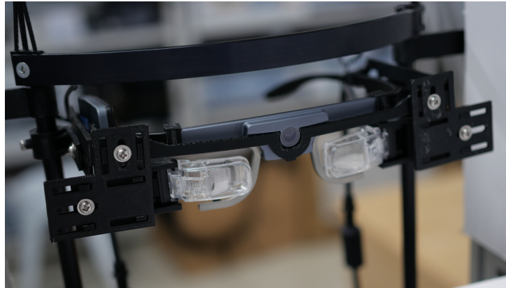
Figure 6.18 – Close-up of the custom binocular headset with its two RPD modules mounted on an eye tracking device.
