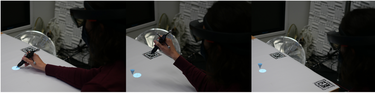
Figure 7.3 – Interaction techniques: direct interaction (left), indirect pointing (middle), gaze pointing (right).
