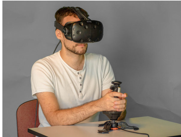
Figure 4.1 – Experimental setup used in all our experiments. Participants were seated on a chair, wore a HTC Vive HMD and headphones. They grabbed a joystick, which was fixated to the table, with both hands.
