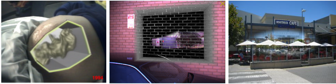
Figure 2.6 – Examples of visualization techniques using x-ray vision: virtual hole, from State et al. (1994) (left), edge-based representation, from Avery et al. (2009) (center), and saliency-based representation, from Sandor et al. (2010) (right).
