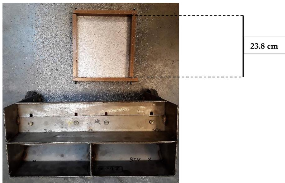
Figure 50. Device for the aggregate spreading.
