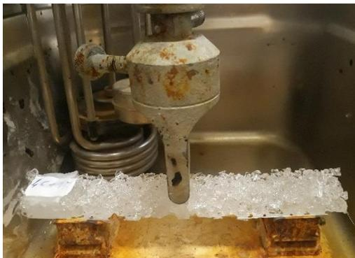
Figure 40. The three-point flexural test.
