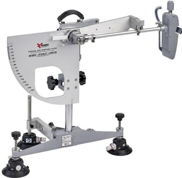
Figure 86. Example of British pendulum test [209].
