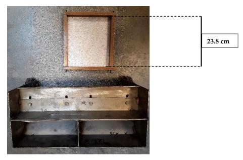
Figure 50. Device for the aggregate spreading.
