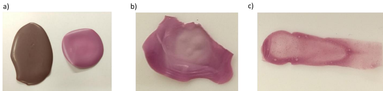
Fig 2.50) [\text{Fe}(\text{HB}(\text{tz})_3)_2](\mathbf{8})@P(\text{VDF-TrFE}) composites obtained by various synthesis conditions. a) Film prepared in DMF (left) and in 2-Butanone (right). b) Film prepared at high viscosity and high thickness. c) Film prepared at high temperature (105°C).
