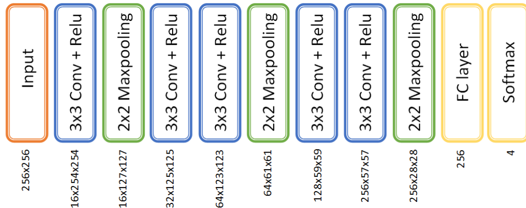
Fig. 57: Architecture of the CNN model. The input layer accepts B-scans with 256x256 pixels from CUHK dataset. The parameters (feature maps and size) are reported beneath every layer.
