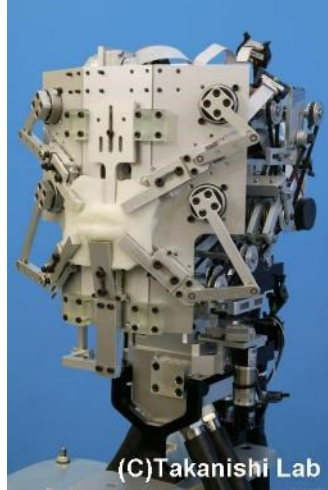
Figure 28 : Photo du robot Waseda Talker (modèle WT-7R11) http://www.takanishi.mech.waseda.ac.jp/top/research/voice/index.htm
