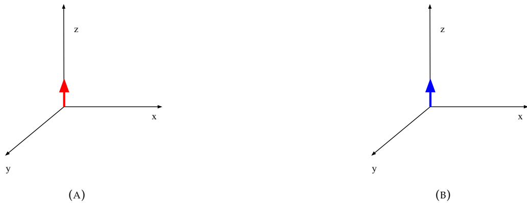
FIGURE 1.5: Diagram representation of infinitesimal electric (A) and magnetic (B) dipoles oriented on the z axis.
