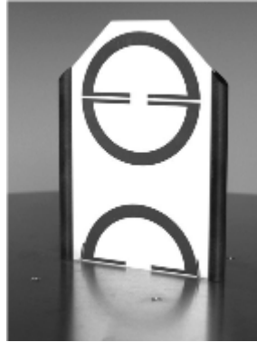
FIGURE 4.7: Magnetic-loop based end-fire superdirective arrays from [20]
