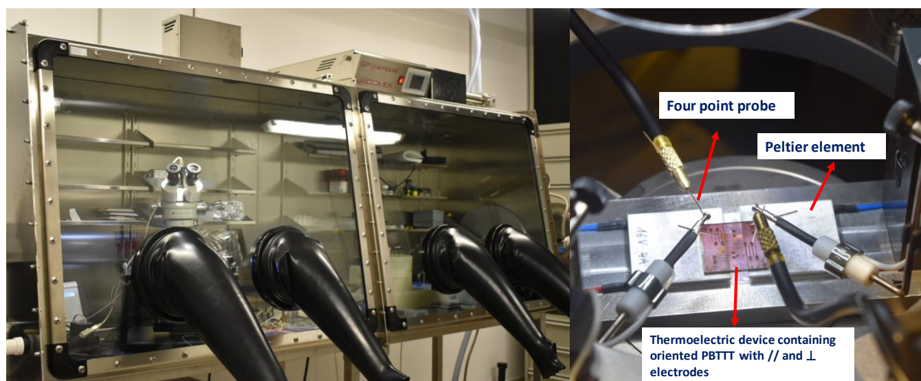
Figure 3. Photographic images of the glove box, electrical conductivity and Seebeck coefficient measurement setup.
