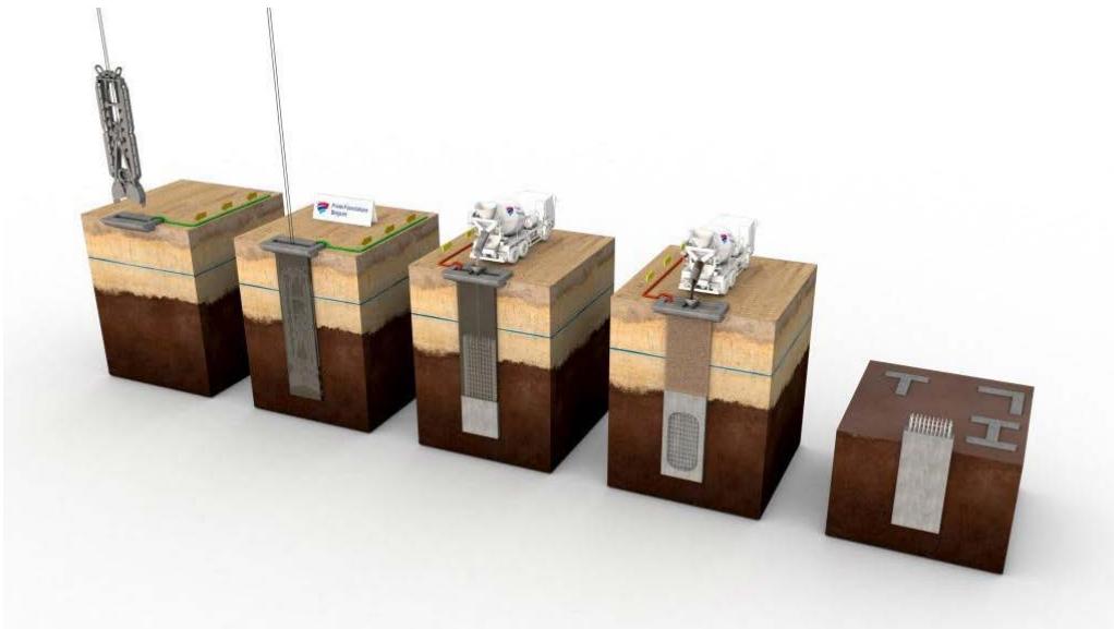
Figure 2-55 : The five phases to realize a diaphragm wall, from left to right.
