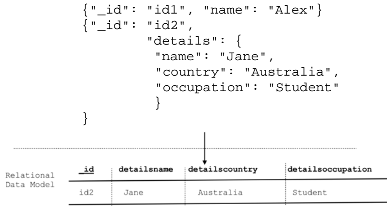
Figure 2.6: Physical re-factorisation of a document data model to relational data model.
