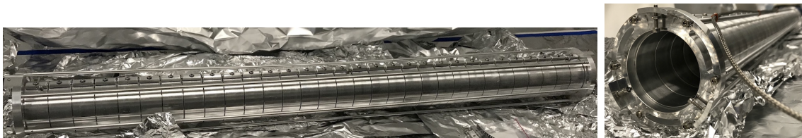
Figure 4.26 – Pictures of the new electron repeller. The repeller is composed of a set of electrodes connected with resistors. The connection to the power supply is made at the center and the electrodes at the extremities are grounded.
