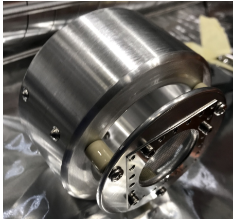
Figure 4.19 – Picture of the electron repeller. A negative potential is applied on the grid to repel the electrons.
