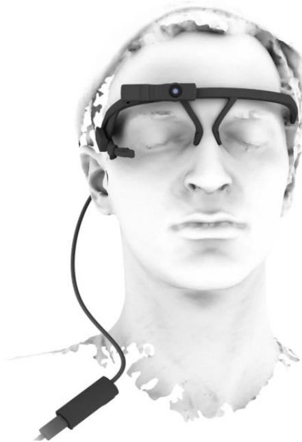
Figure 14. Eye-tracker monoculaire Pupil Labs. Tiré de : https://docs.pupil-labs.com/ ©PupilLabs
