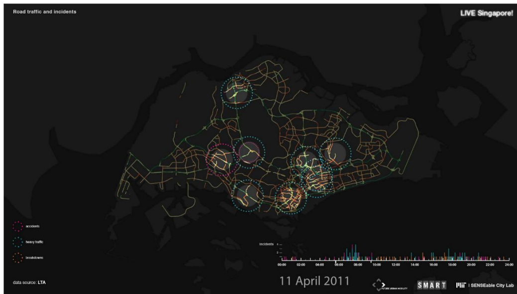
Figure 2.2.11: Visual interface to explore the propagation of traffic congestion. The circles clear the locations where an incident occurred revealing the traffic conditions. The temporal variation of traffic can be explored via a timeline that gives the intensity of traffic incidents over time (bottom right). Source: Anwar et al. (2014) .
