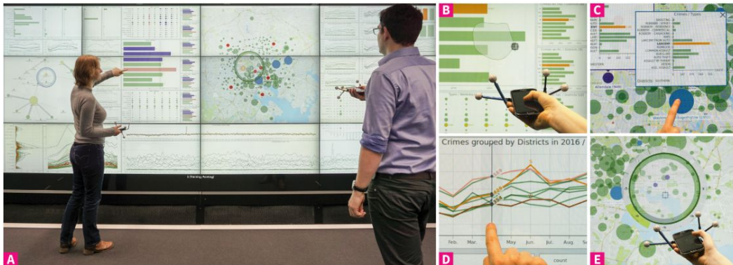
Figure 2.3.1: Multi-user CMV application on an interactive wall-sized display: (a) Interaction from close (touch) and distance (mobile device); (b) Data selection; (c) Details on demand; (d) Interactive ruler for value comparison; and (e) Magic lens with menu. Source: Langner et al. (2018).
