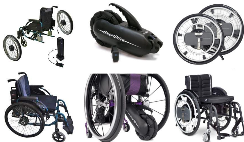
Figure 2.2.1. Duo kit, Smartdrive and Wheeldrive commercialized respectively by Autonomad Mobility, MAX Mobility and Sunrise Medical (From left to right)
