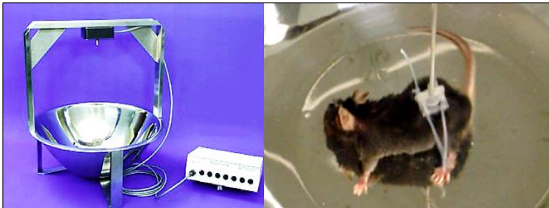
Figure 31: The apomorphine-induced rotation test. Following 6-OHDA lesion in the left SN, apomorphine injection triggers a rotation behavior in an opposite direction to the lesioned side. The mouse in the bowl is attached to a rotometer head by a harness so that ipsilateral and contralateral turns are assessed by the automated rotometer system.
