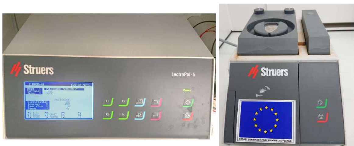
Figure 2.11. Struers LectroPol-5 system with electrochemical polishing parameters shown in on the screen.
