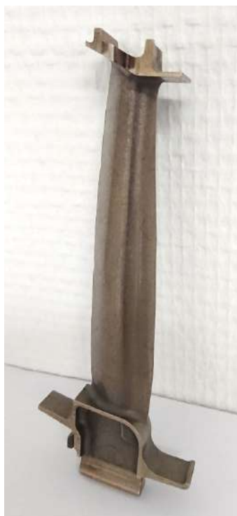
Figure iii. An example of a non-cooled first stage LPT blade
