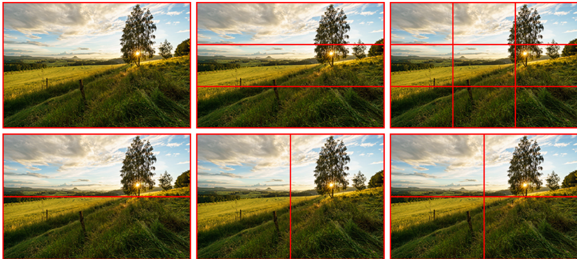
FIGURE 2.23 – Illustrations of region splits. The first row shows the whole scene and regions split by landscape rule and rule of thirds respectively. The second row presents regions split by symmetry rules.
