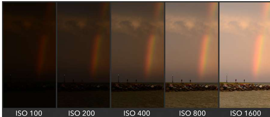
FIGURE 2.21 – Pictures taken with different ISO modes. When increasing ISO, the camera sensor is more sensitive to light and the photo looks brighter (image source : https://photographylife.com ).
