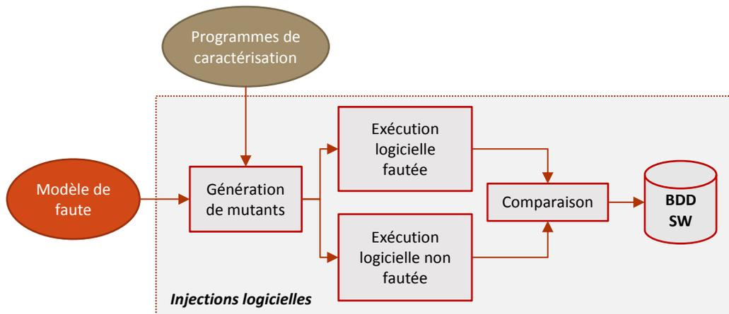
**FIGURE 37 : VUE D'ENSEMBLE DE L'INJECTION LOGICIELLE. LES PROGRAMMES DE CARACTERISATION SONT UTILISES DANS DES EXECUTIONS FAUTEES ET NON FAUTEE. LES RESULTATS SONT COMPARES ET STOCKES DANS UNE BASE DE DONNEES**
