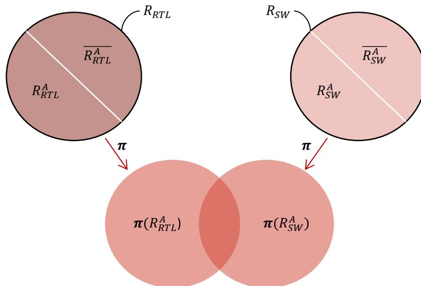
**FIGURE 39 : REPRESENTATION DU RECOUPEMENT DES COMPORTEMENTS RTL ET LOGICIELS. LE CERCLE EN HAUT A GAUCHE REPRESENTE LES RESULTATS D'INJECTION RTL ET CELUI EN HAUT A DROITE, LES RESULTATS D'INJECTION LOGICIELLE. CES DEUX CERCLES PEUVENT ETRE DIVISES EN FAUTES ANALYSABLES ET NON-ANALYSABLES. LES PARTIES ANALYSABLES PEUVENT ENSUITE ETRE PROJETEES VERS L'ESPACE DES COMPORTEMENTS POUR ETUDIER LEUR RECOUPEMENT.**
