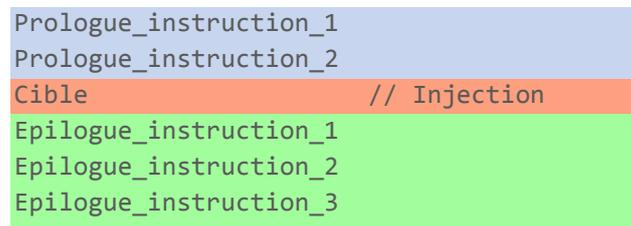
**FIGURE 30: STRUCTURE D'UN PROGRAMME DE CARACTERISATION**
