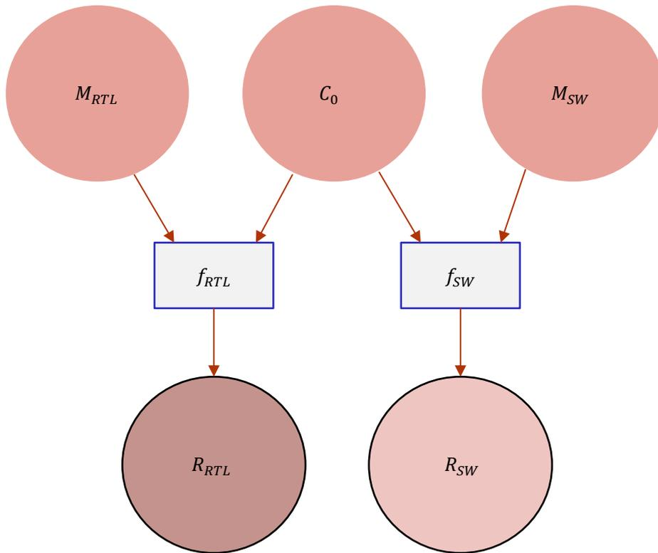
FIGURE 38 : DIAGRAMME DES CAMPAGNES D'INJECTION DE FAUTES. LES INJECTIONS AU NIVEAU RTL,  $f_{RTL}$ , PRENNENT EN ENTREE LES BASCULES A FAUTER  $M_{RTL}$  ET LES PROGRAMMES DE CARACTERISATION DE  $C_0$ , ET GENERENT LES RESULTATS D'INJECTION  $R_{RTL}$ . DE MEME, LES INJECTIONS AU NIVEAU LOGICIEL  $f_{SW}$  PRENNENT EN ENTREE LES MEMES PROGRAMMES DE CARACTERISATION DE  $C_0$ , AINSI QUE LES MODELES DE FAUTE DEFINIS DANS  $M_{SW}$  POUR PRODUIRE DES RESULTATS D'INJECTIONS  $R_{SW}$ .
