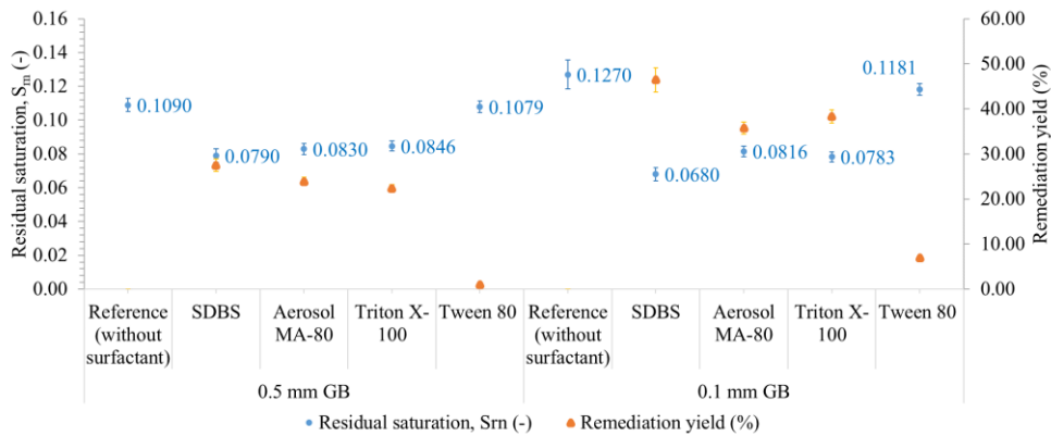
Figure 112: S_{rn} and remediation yields with the four surfactants with 0.5 and 0.1 mm GB (average values at the end of imbibition 1)
