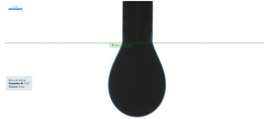
Figure 48: Digitized pendant drop during the measurement of IFT
