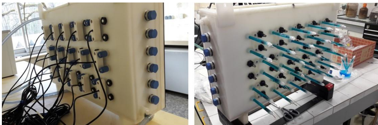
Figure 199: Photograph of the geophysics measurement (TDR and resistivity) tools network on the back of the 2D tank
