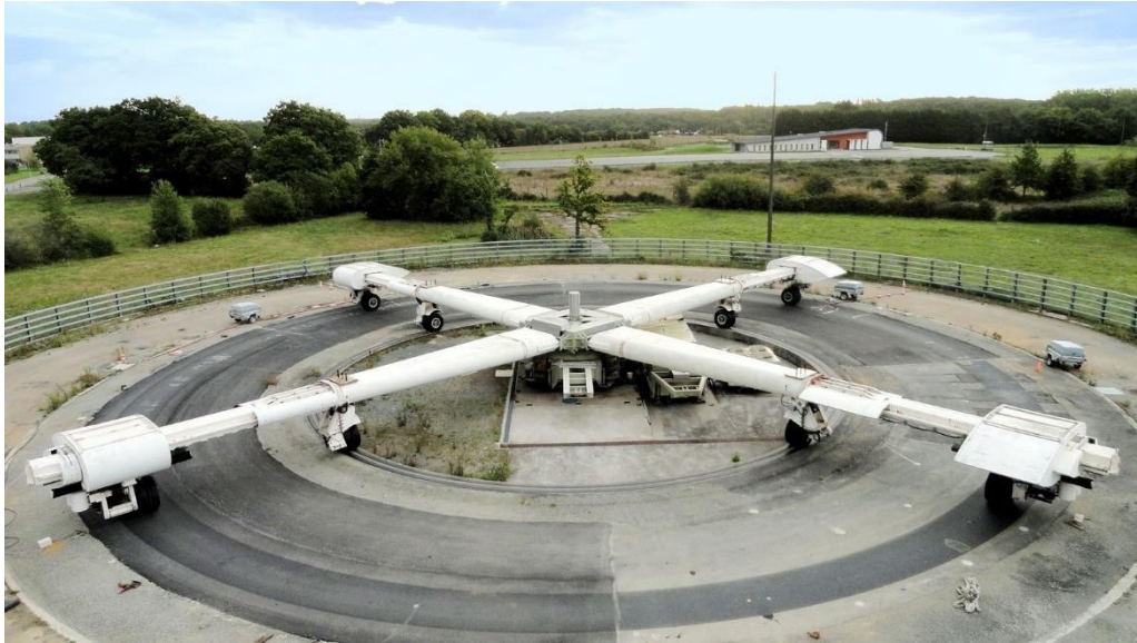
Figure 2.1 The University Gustave Eiffel fatigue carousel: four arms are controlled by a central electro-hydraulic motor unit. The perimeter is 120 m long.
