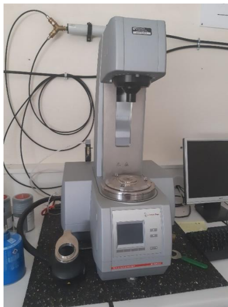
Figure 6.11 DSR device EC-Twist 502 manufactured by Anton-Paar at the Eiffage Route Research Centre. Table 6.2 Temperatures and frequencies used for DSR complex modulus test on the bitumen of the tack coat emulsion.
