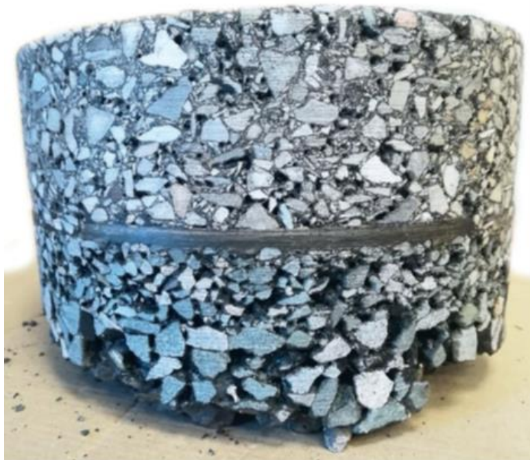
Figure 3.9 Sample cored on the trial section 2 months after the installation: very good bonding at the interfaces InTrack/asphalt.
