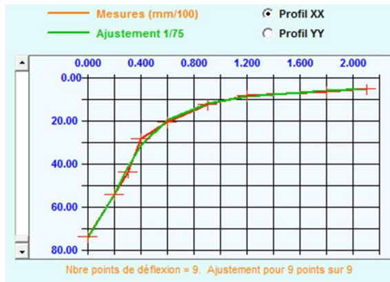
Figure 2.27 Results obtained in Alizé by performing an inverse calculation from the measured basins representative of the damaged zone: (left) Mix3, (right) EME2. The measured basins are well predicted by the model.
