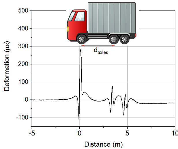
Figure 3.21 Example of a signal collected during the campaign of measurements. Knowing the geometry of the passing truck, the actual speed can be determined with the time interval of the two peaks caused by two axles. The abscissa x = 0 m identifies the passage of the front axle.
