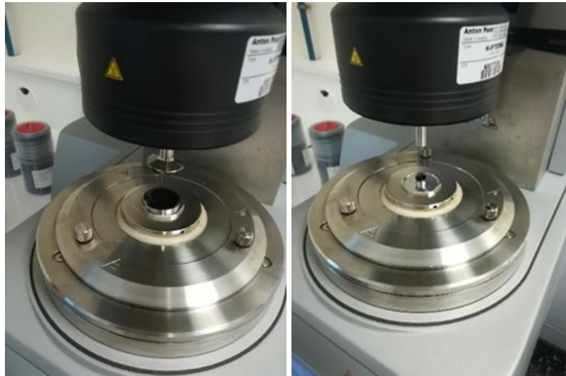
Figure 3.11 Samples used to perform the complex modulus test on the bitumen of the tack coat emulsion: (Left) 25 mm test sample; (Right) 8 mm test sample.
