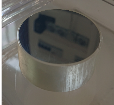
Figure 4.18 – A 10 \mu\text{m} Al film evaporated on one side on big LMO.
