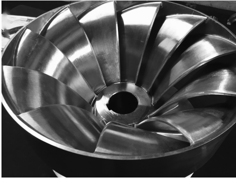
FIGURE 1.2 – Roue de turbine Francis
