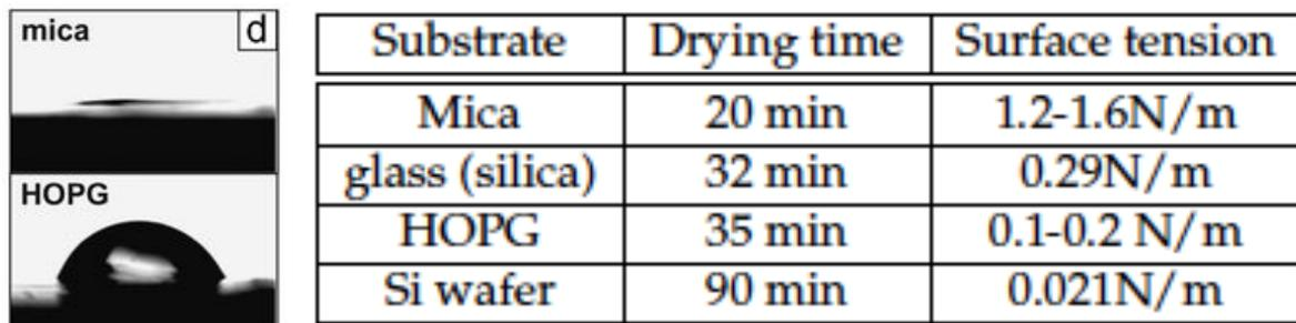
**Figure 66. Different form of droplets with water as solvent and drying time depending on substrate.**
