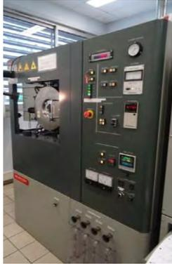
**Figure C-1 :** Machine SPS Syntex Inc. Dr Sinter 2080.
