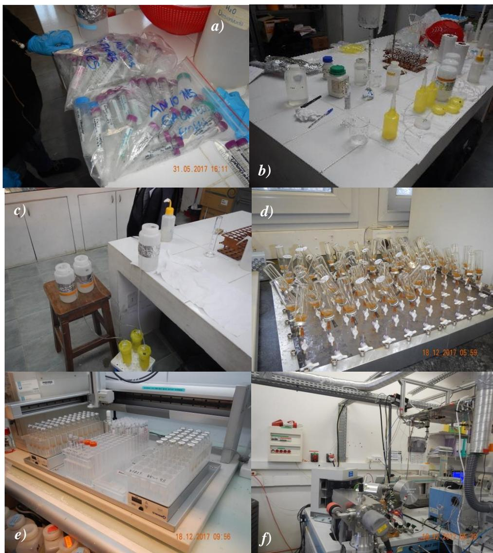
**Figure 3.9.** a) Samples for major ion analysis, b) materials for the preconcentration procedure, c) Samples (1 liter) were poured in the funnels and drained by gravity, d) preparation of the 10 ml eluted samples by the addition of bacteria in order to ensure 100 nmol of  $\text{NO}_3$  and a matrix volume of NaCl, e) 12 hours of incubation, then NaOH was added for trapping nitrogen dioxide in each vial, and finally isotopic compositions were measure in the f) MAT 253 IRMS Mass Spectrometer.
