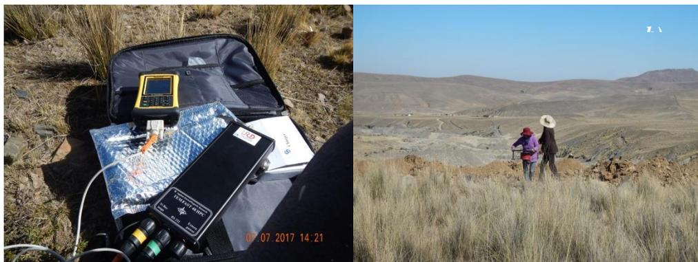
**Figure 3.6.** a) TEMfast 48 equipment used for measuring resistivity parameters in the field and b) Example of setting the coincident loop configuration in the field.
