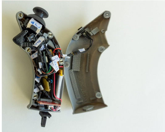
Figure 2.21: A specially designed input device CHARM [Klamka et al., 2019] for AR manipulation.
