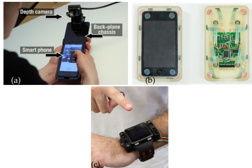
Figure 5.6: Examples of using complex setups to augment tactile input: (a) the combination of tactile input with in-air gestures by Chen et al. [2014]; (b) combines tactile input with pressure using a self-designed unit [Heo and Lee, 2012]; (c) uses gestures to augment tactile input [Withana et al., 2015].
