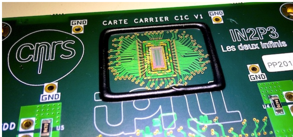
Figure 4.15: Wire-bonded CIC1 on the carrier board.
