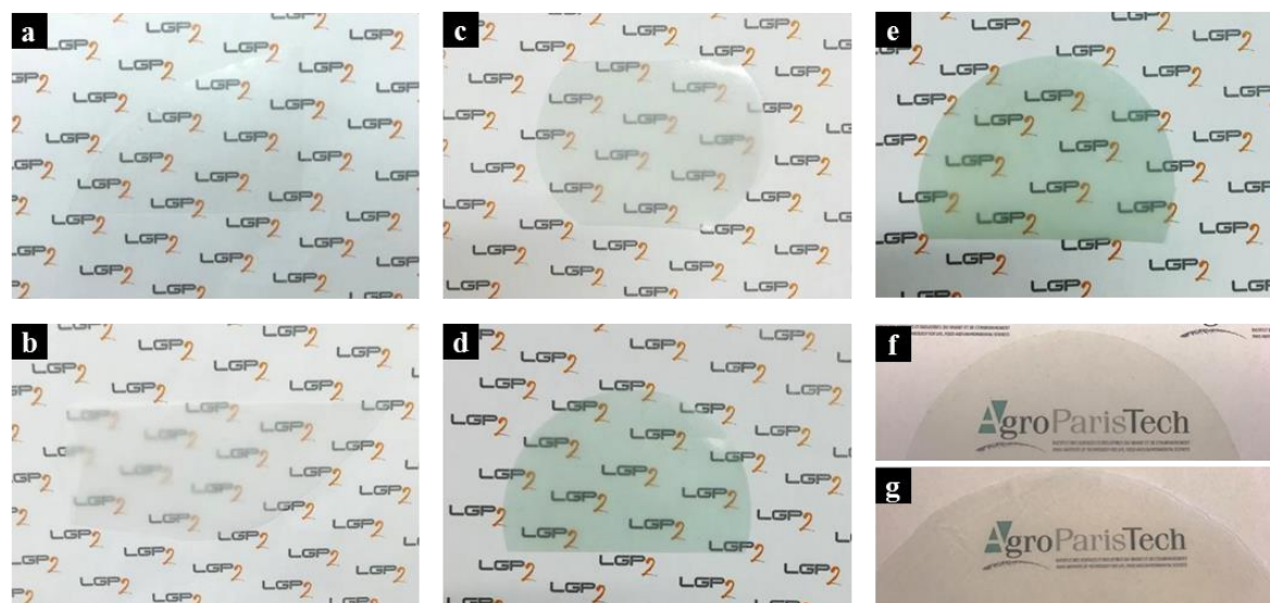
Figure III. 2. Photographs of a) neat PLA casted film, b) PLA_neatCNC10 nanocomposite, PLA_CNC-PGMA-Br nanocomposites with c) 2 wt%, d) 5 wt%, and e) 10 wt% of polymerized CNC-PGMA-Br, and PLA_CNC-Lauric nanocomposites with f) 5 wt% and g) 10 wt% of modified CNC-Lauric
