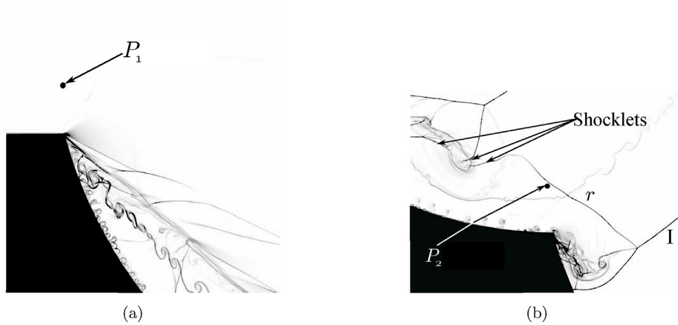
Fig. 10. Numerical schlieren pictures for M_s = 4.5 at t = 69 \mu s : (a) beginning of the first concave surface; (b) beginning of the second concave surface; I: incident shock wave; r : reflected shock wave, P_1 and P_2 are two probes locations.
