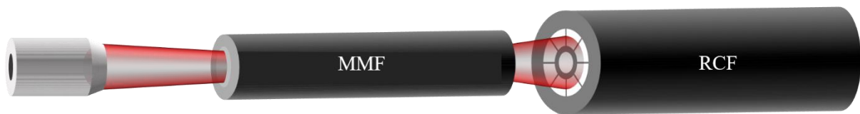
Figure 77 Schematic illustrating the principle of RCF excitation using a MMF.
