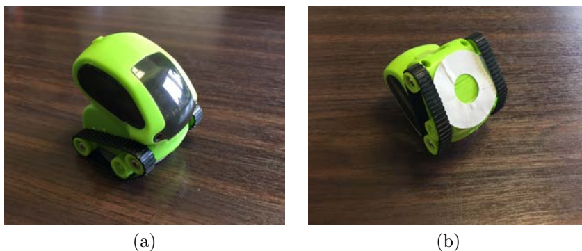
Figure 5.1: (a) Mini-robot toy used on the tabletop surface, equipped with RFID tags. (b) The RFID tag stuck to the mini-robot from below, used on the tabletop surface.
